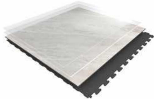
**Design Tile** is a synthetic, decorative, flexible, antistatic, abrasion group T floor covering. It consists in a multi-layered tile with a 0,70 mm thick transparent wear layer and a printed film on an injected molded backing. The overall thickness is 7,8 mm.
